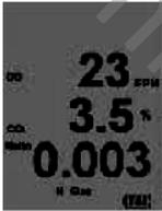
The top display shows the carbon monoxide level.
