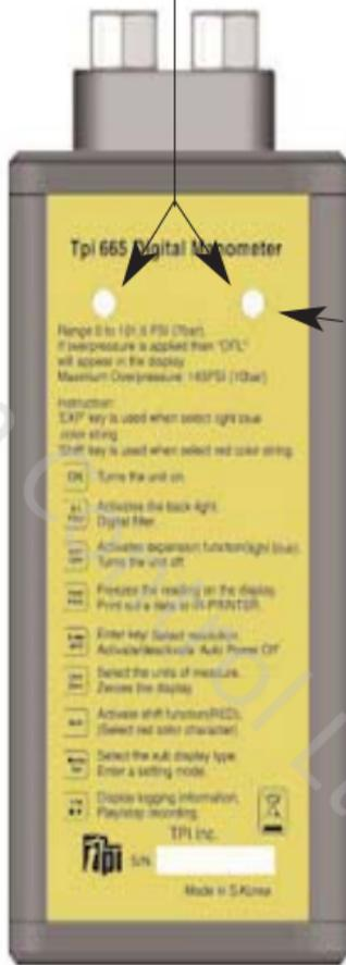
IR Port for printing using optional A740 printer
