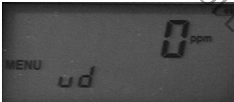
“0ppm ud (ud=under)” will display leaks in steps. The steps are 0ppm, ud 500ppm, ud 1000ppm, ud 3000ppm, ud 5000ppm, ud 9999ppm
