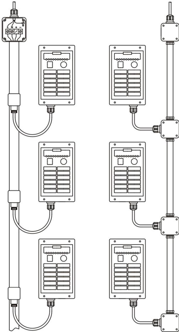
TraxBus using busbars or single wire lines
