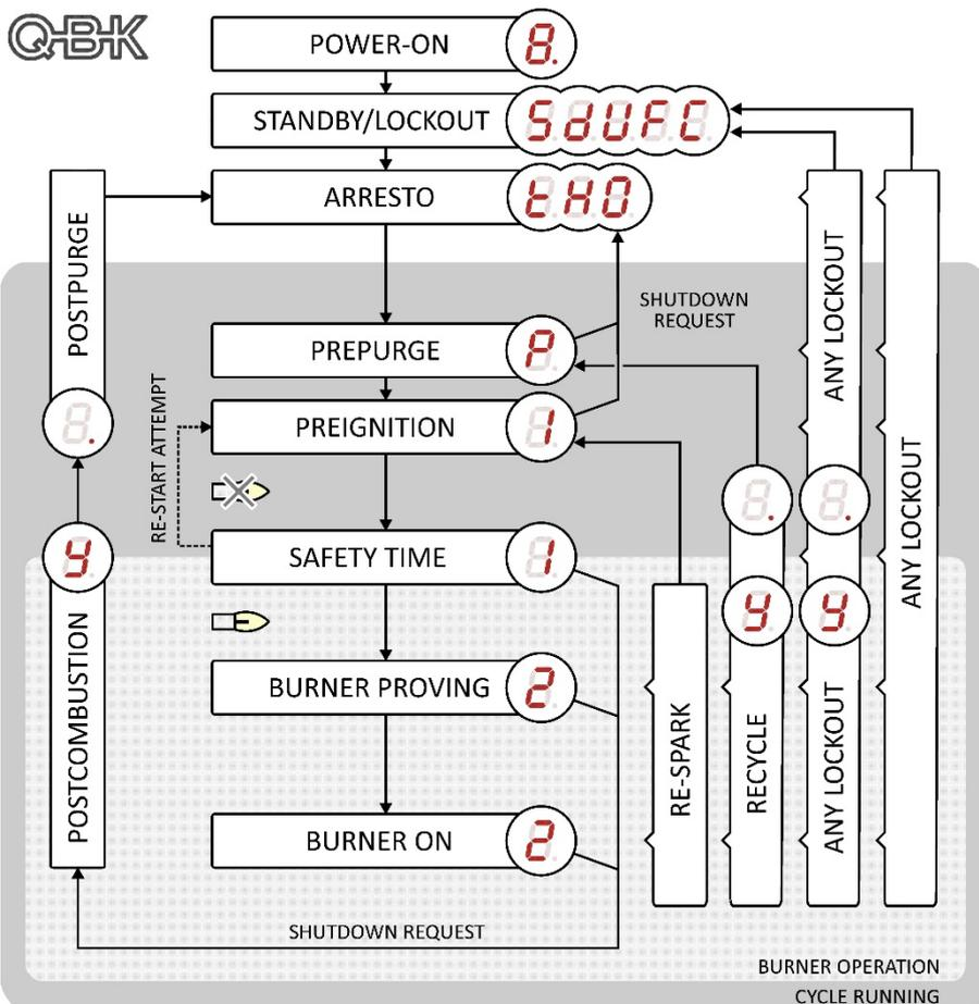
A **SELF TEST** IS PERFORMED AT POWER-ON, ONCE SUCCESSFULLY COMPLETED BURNER IS READY TO START.
