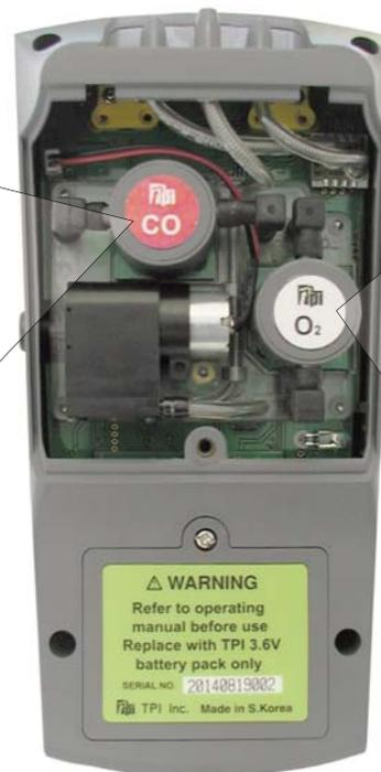
Smart sensor access panel removes with the turn of a screw and provides ample working room for sensor replacement.
