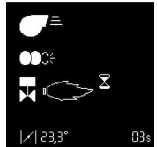
**If no flame is detected at the end of the safety time**, the control unit switches to malfunction mode.
