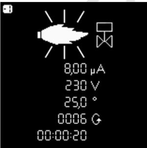
Using the buttons and , it is possible to call up the details of the last 5 faults to have appeared (the fault number is displayed in the upper left corner of the display). After the details of the last 5 faults, the telephone number of the after-sales department as well as the maintenance contract number are shown (no values are entered in the factory).
