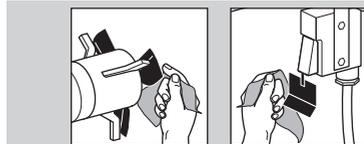
13 Check that the vane switch is functional.
