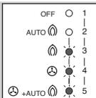
! While a fault was pending, more than 5 attempts were made within 15 minutes to reset the device using the remote reset input (terminals 31 and 32).
