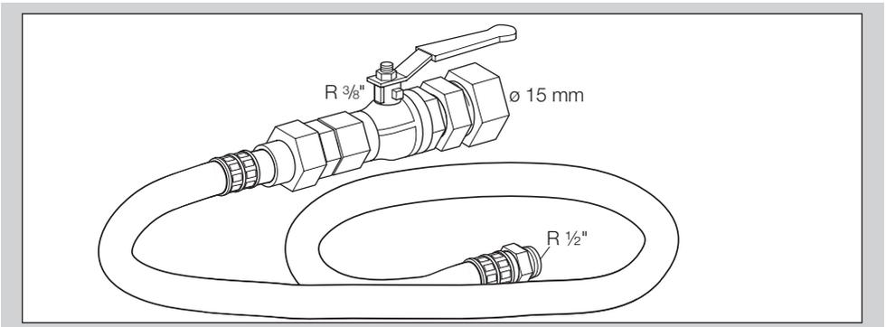
Manual valve and hose (DVGW certified, length = 2 m) to connect the gas combination control CG to the gas supply, Order No.: N52990209
