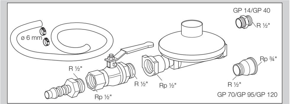
Pressure reducer, manual valve, hose (length = 2 m), 2 hose clamps, R 1/2" double nipple for GP 14/GP 40, R 1/2 - Rp 3/4" reducing fitting for GP 70-GP 120, to connect the gas combination control CG to the gas supply, Order No.: N52600025
