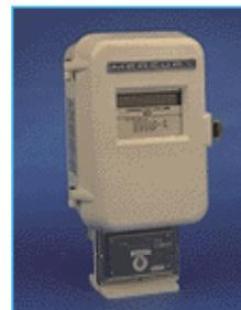
Most instruments come with Mechanical Uncorrected Pulse Output. This is generated by a magnet on a drive shaft from the instrument's Mechanical Uncorrected Index (UMB) passing a reed switch. There should be a terminal block on the Meter Pulse (or Switch) Board that facilitates wiring to this pulser. (see Diagram 1, or page 13, sec 6.10 and Page 58, sec. 11.1 of Mercury Mini User's Manual)
