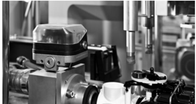
Monitoring the negative pressure ensures the correct positioning of the components during fully automatic assembly of gas meters.
