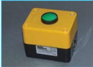
A push button operated switch which isolates the electrical supply to the valve in the event of power failure. When power is restored to the valve, the push button must be depressed before the valve will open. Integral and remote versions are available. Suitable for screw fixing to a flat surface. Route electrical supply to valve through unit; electrical connection via screw terminals, cable entry 20mm diameter.
