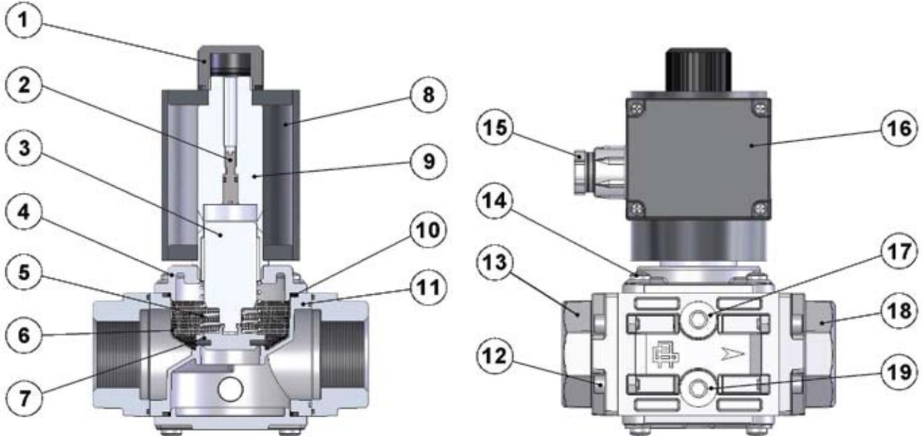
Fig.3 - Series 2000 Component Parts
