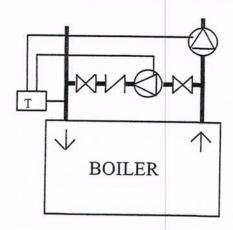
To eliminate totally the problem, it should make perfect the above mentioned design to maintaining the temperature of the boiler (55 °C) also by night and add a further temperature limit fuse thermostat tha operate to the unit mixer valve not forward to the boiler, water not at 55 °C.
