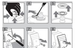
Remove the M20 cable gland or other type of connection.
