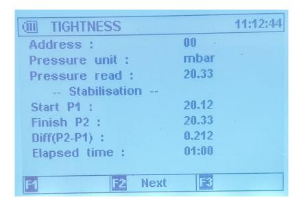
Press the "F2" Key to move onto the Tightness section of the test.
