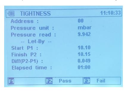
Press the "F3" Key to Fail the test or
