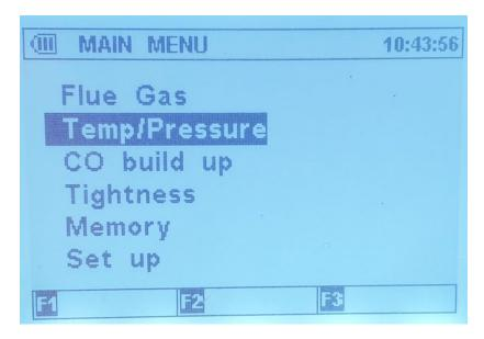
On this screen you can view the Temperature in T1, T2 and the differential between both as well as the Live Pressure.
