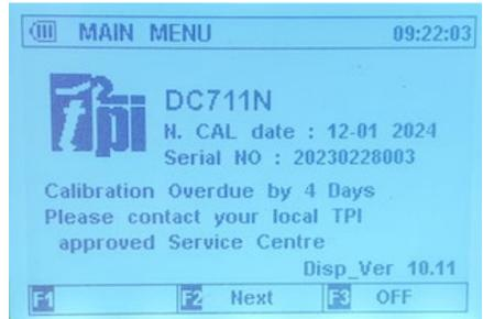
Choosing "Next" will move you onto the Main Menu Screen as displayed below. **Please Note:** In the UK, it is a requirement of BS7967 that an FGA is within calibration and used in conjunction with the manufacturer's instructions therefore it is NOT recommended that "Next" be chosen by the user if the Calibration is Overdue. Doing so will contravene the requirements of BS7967.
