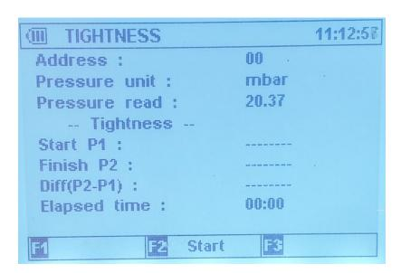
The test continues with the Tightness section so please apply the required pressure which will be displayed as "Pressure read" value.
