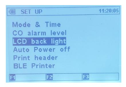
Entering "LCD back light" will display the following where you can adjust the LCD backlight level. Higher levels of backlight will reduce battery life.
