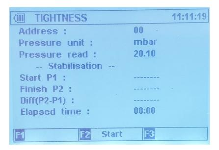
Press the "F2" Key to Start the Stabilisation section of the Test
