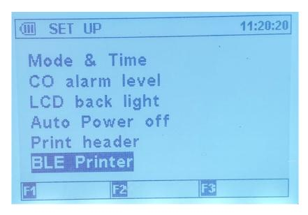
Entering "BLE Printer" will display the following where you can scan and pair available optional A741BT Bluetooth Printer to your DC711.
