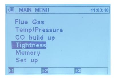
Press the "F1" Key to Zero the pressure, if required, before attaching the pressure hose.
