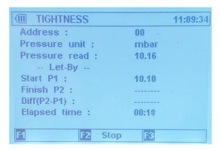
Once the 60 seconds have elapsed the Start, Finish & Difference pressure will be displayed with option for you to Pass or Fail the test at this stage.
