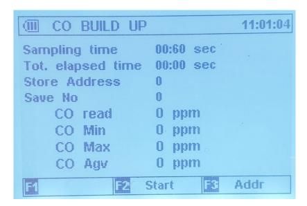
At any time during the test, you can press the "F2" Key to Stop the Test.
