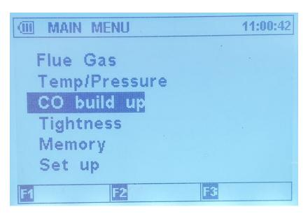
Entering the CO Build Up function will start the Purge Period. During this period you can press the "F2 Key" to skip, if displayed.
