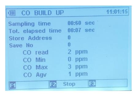
As long as the test has run for longer than 60 seconds the report will be available to Print immediately by pressing the "F1" Key or be saved automatically to the chosen Storage Address for output later.
