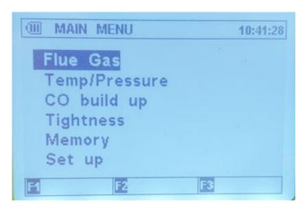
If this is the first time you are turning the DC711 on, we suggest you head over to the "Set-Up" section to investigate the options as described below. Press the Up or Down Arrow Keys, to highlight "Set up" then press the "Enter" key.
