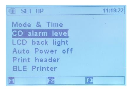
Entering "CO alarm level" will display the following where you can toggle the ambient and High CO alarms On & Off, as well as adjusting the default levels to suit your testing requirements
