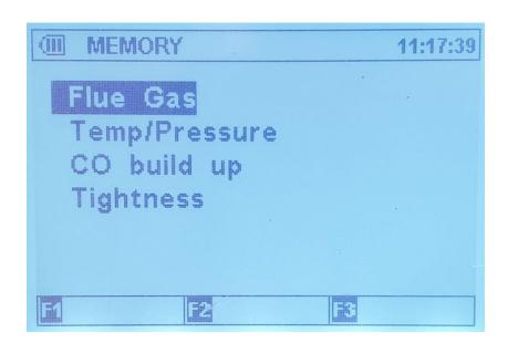
Once the section required is Highlighted use the Enter Key to bring up the Memory options.
