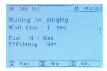
Once the Purge Period is complete the DC711 will display the Gas Test Screen including NO and NOx (if fitted).
