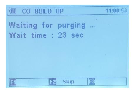
Once the Purge Period is complete the following screen is displayed where you can start the Ambient Air CO Build Up Test.
