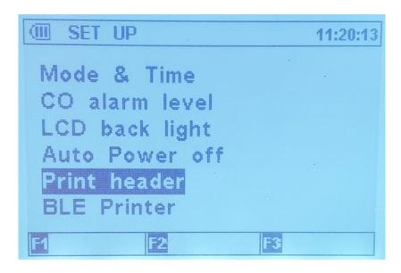
Entering "Print header" will display the following where you can add or edit the details that will print out at the top of each report when using the optional A741BT printer and direct printing from the analyzer.
